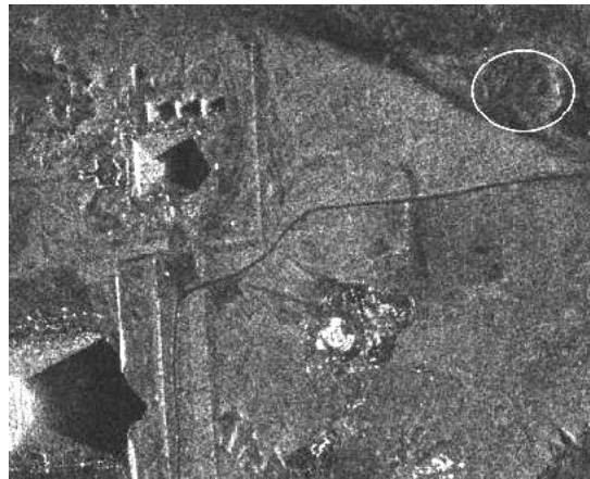
Fig. 15 Terrasar-X Uncovers the Wall of the Moon Credit: DLR; date: July 2, 2007, 03:47 UTC; original resolution: 1 metre (reduced image); mode: High Resolution Spotlight Mode; polarisation: HH
