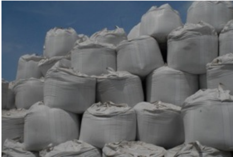
Fig. 8 Stack of cement sling bags each weighing about 3 tons
